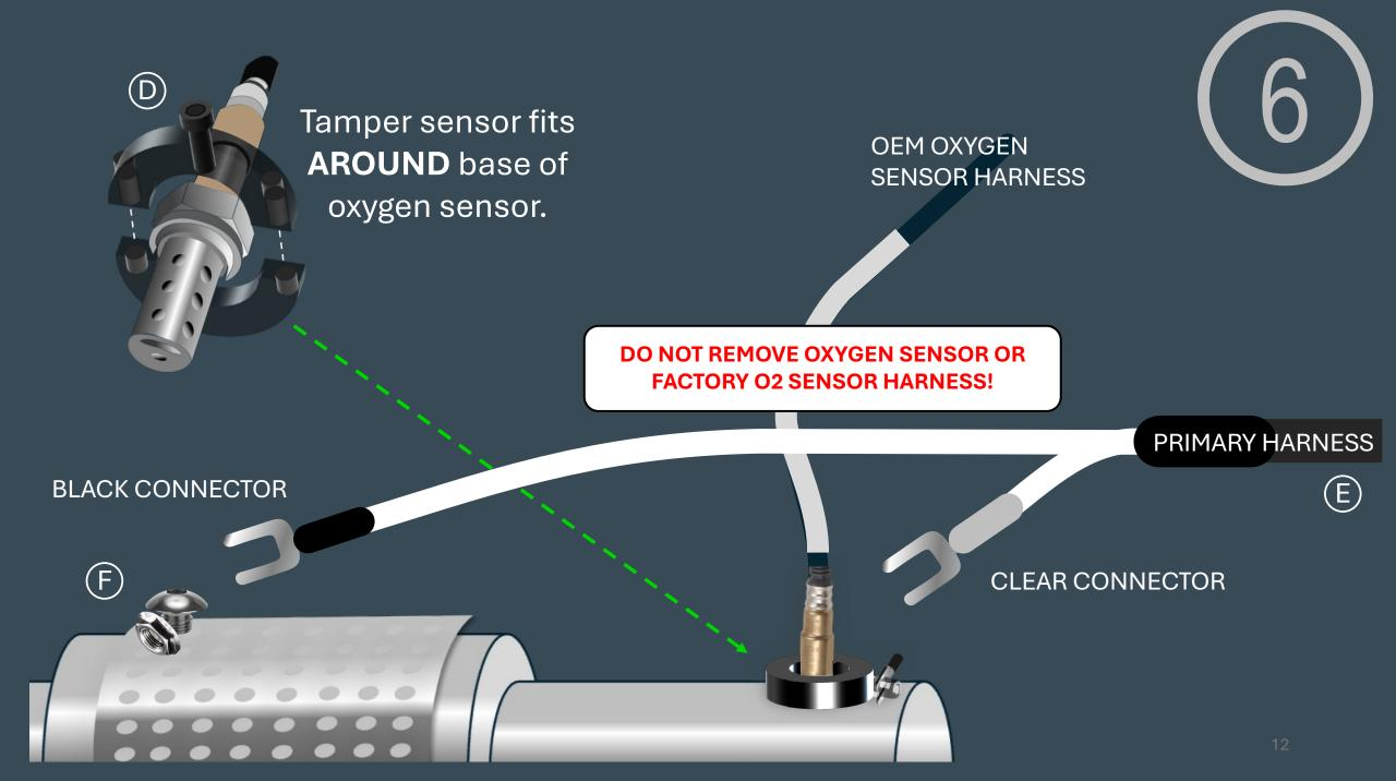
Creating a quality chassis ground is extremely important. There are two connections that are required on the exhaust/catalytic converter. The black fork connector is applied toward the rear of the exhaust with the clear fork connection attached to the tamper sensor. If there is no heat shield, use the exhaust flange stude or posts.
