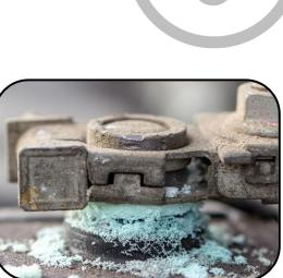
Inspect battery terminals for corrosion, clean terminals prior to installing ring terminals if needed.
